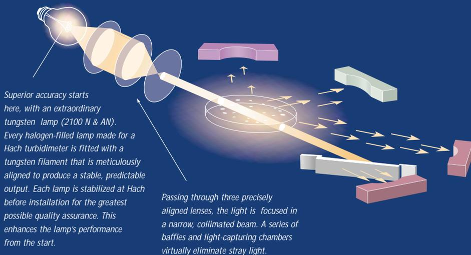
With a back-scatter detector, 2100AN and 2100AN IS models are uniquely equipped to measure high levels of turbidity (up to 10,000 NTU) with excellent accuracy.
